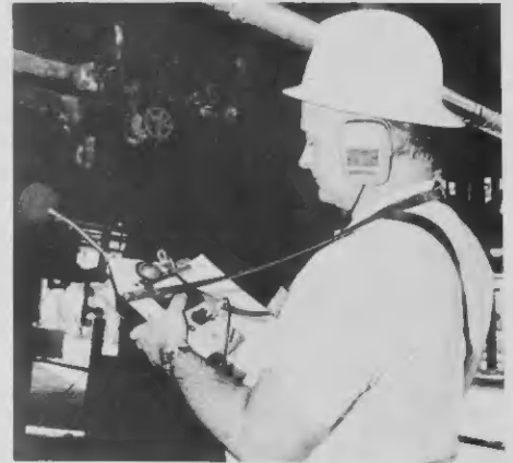
Tom Bragg employs sensitive instruments to measure and record noise levels in work areas in the refinery.
